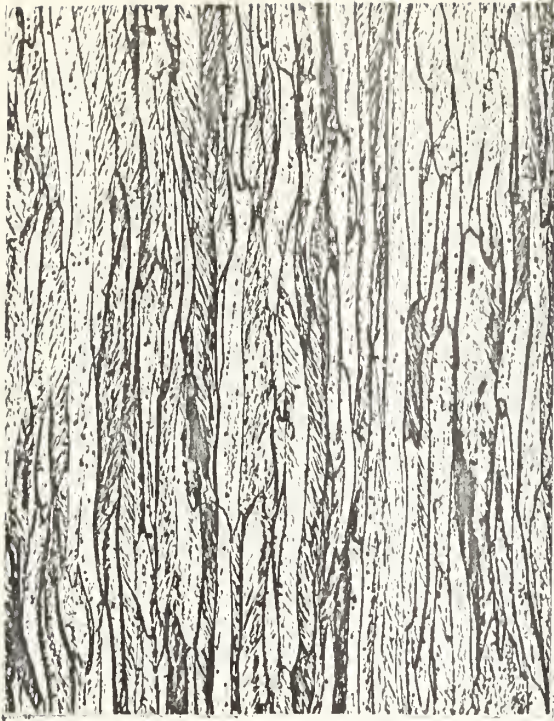
FIG. 5 AS ROLLED CONDITION (ROCKWELL 30T 70)
